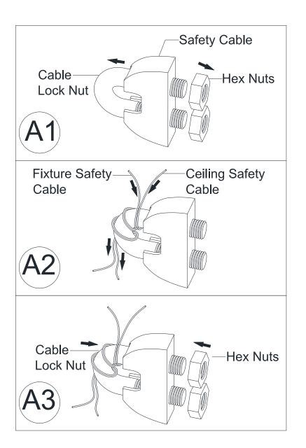
1. Remove Hex Nut from Cable Lock Nut and pull Cable Lock Nut from Safety Cable.
