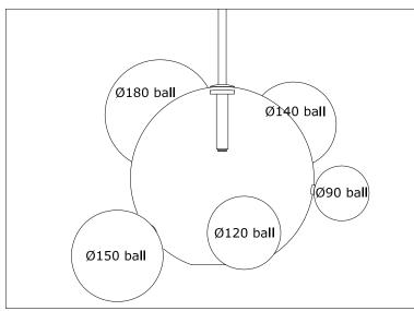
STEP 7: Assemble the LED light source(P,2x3W,3000K) into the fixture body(T) from bottom of the biggest glass ball.
